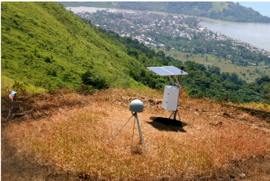
Figure 11. GPS station at Air Bangis, West Sumatra, with the coastal community of Air Bangis in the distance.
